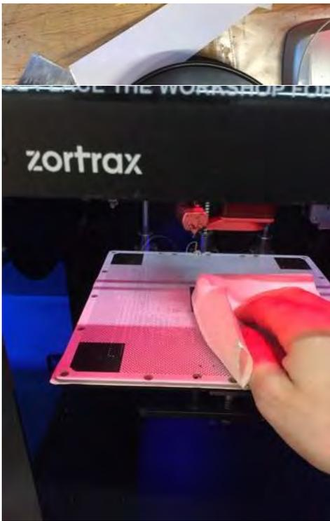
Ensure that the print bed is clean – remove any residues from earlier prints and wipe it with ethanol.
