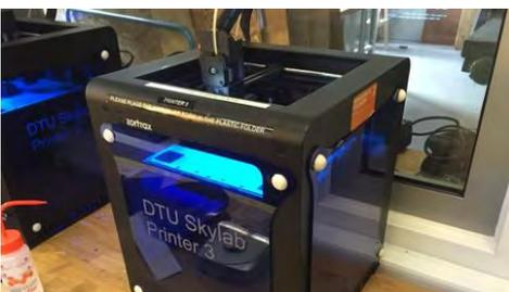
Place all side covers on the printer when in operation and do not put an open ventilation nozzle close to the printer (it creates a draft which introduces stresses to the print).
