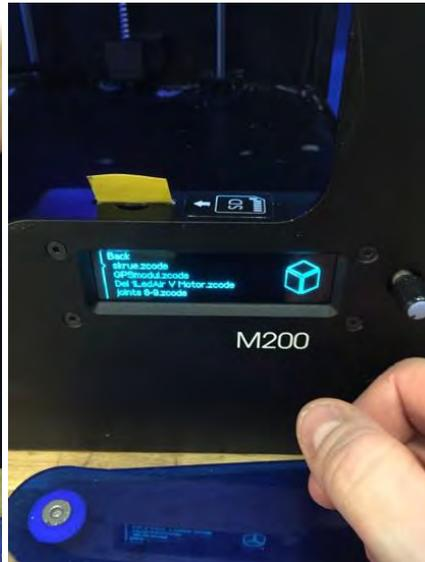
Use the knob to navigate the printer menu. To start a print simply chose 'models' and select for file (usually the top-most one).
