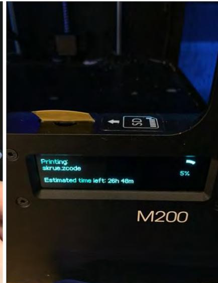
The printer starts when it has finished heating the hot-end and print bed. The display shows the process and time remaining.
