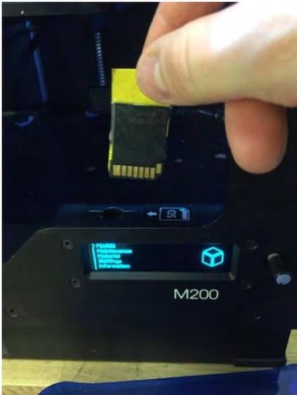
The SD card (with your g-code on it) is inserted into the printer. Orient the card so that the connection pins are pointing towards you.
