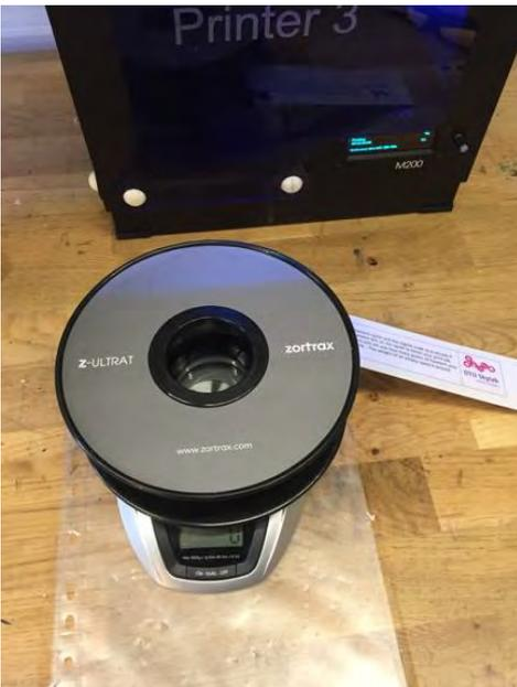
Ensure that there is enough filament left on the spool. If you are in doubt you can use the scale on the desk and check the weight of the spool (the spool itself weighs around 100 g). Z-suite provides you an estimate of filament consumption in grams (and print time) use this information to see is there is enough filament.
